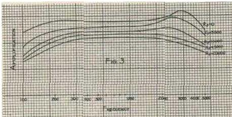
Fig. 3. The effect of plate impedance on the operation of a transformer of high primary impedance. The curves of Fig. 2 and 4 show the importance of making measurements with a resistance in series with the transformer primary. Otherwise an entirely false impression may be conveyed.
