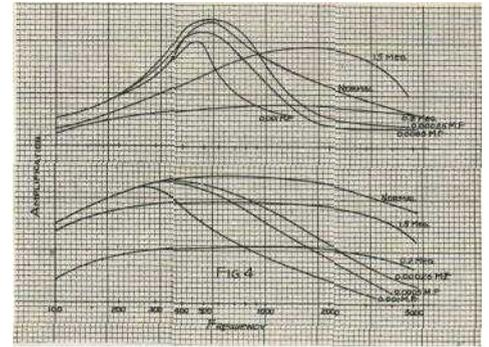
Fig. 4. A group of curves showing the effect of shunting various devices across the transformer secondary. The upper group were taken with a poor transformer, the lower on the newer types.
