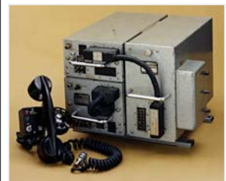
Figure 1 The mobile unit for MTA, the world's first automatic mobile telephone system.
