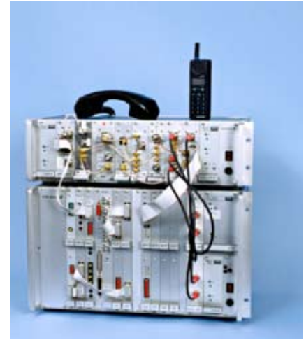
Figure 3 Two versions of the first GSM mobile phone: prototype and commercial handset.
