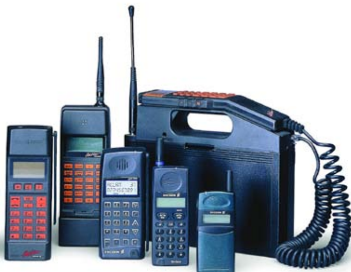
Figure 2 The size of mobile handsets quickly diminished between 1981 and 1998 thanks to rapid advances in microelectronics and digital technology. In particular, GSM gave rise to pocket-sized mobile phones.
